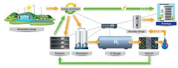
The SAGES® station is controlled by an E.M.S. (Equipment Management Software), PowiDian Energy's proprietary software, installed in a Master Controller, to manage the equipment locally. An intelligent software layer is added to enable autonomous equipment control decisions (starting, shutdown, optimization of the operating point, alarms, etc.).
